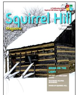
Tony Indovina's 2020 photo of the Neill Log House was featured on the cover of the current *Squirrel Hill Magazine*. The photo shows the urgent need to repair and restore the house to prevent further deterioration. Some of the logs at the bottom of the house are pulling away from the foundation, causing water damage and damage from animals getting into the house.
